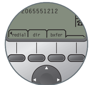
FIGURE 2: When you're on a call, you can press the right arrow on the navigational wheel to see these additional soft key options. The bxfer soft key enables you to transfer a call quickly, rather than waiting to announce the call to the other party, as with the xfer soft key.
