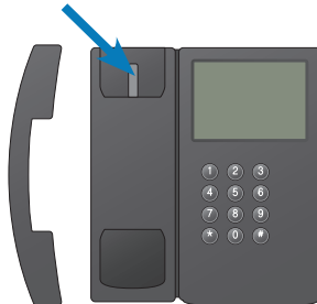
FIGURE 2: This is the hook button . With some phones, you can use a labeled flash button instead.
